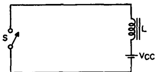
Fig. 85—Simplest form of deflection circuit.
