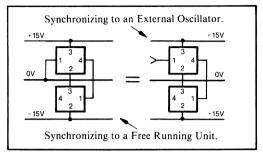
Tha master pin is a buffered output designed to drive other slave inputs. In split rail applications it is recommended that the external oscillator drive only one unit and all others be driven from the master outputs of other PWR1017s.
