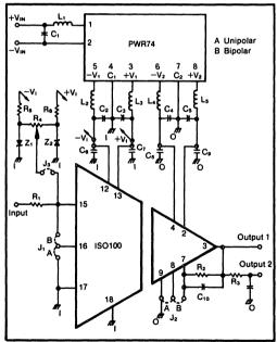
FIGURE 1. Example Circuit Diagram.
