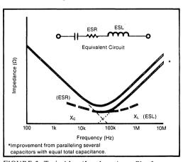
FIGURE 3. Typical Log/Log Impedance Plot for Aluminum Electrolytic Capacitor.
