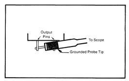
FIGURE 1. Recommended Noise Measurement Method.
