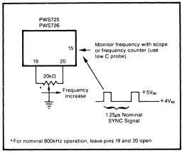
FIGURE 4. Frequency Adjustment Procedure.
