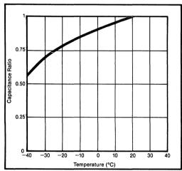
FIGURE 5. Capacitive Ratio Relative to Room Temperature.
