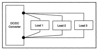
FIGURE 1. Recommended Power Distribution.
