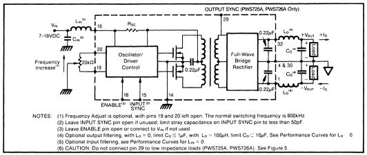
FIGURE 1. PWS725/726 Functional Diagram.
