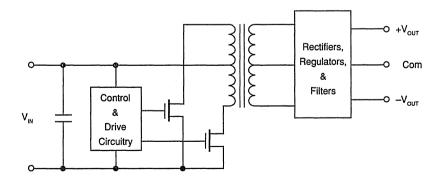
FIGURE 6. Push-Pull Converter.
