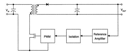
FIGURE 2. The Flyback Converter.
