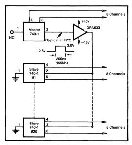
FIGURE 1. Master/Slave Synchronization of Multiple PWS740 Drivers.
