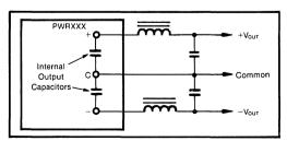
FIGURE 2. Output "PI" Filters.
