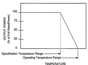
FIGURE 1. Derating Curve.
