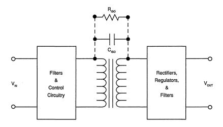
FIGURE 4. Isolation Resistance And Capacitance.
