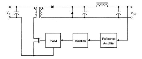
FIGURE 3. The Forward Converter (With Output PI Filter).
