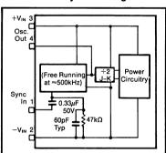
NOTE: Care should be taken when the synchronization input pin is not used, in order to avoid the possibility of noise pick-up and false PLL locking. This could destroy the unit and/or any other units that are coupled to its synchronization output (pin 4). This protection may be accomplished by either tying the synchronization pin to  $-V_{\text{IN}}$ , or clipping pin 1 off flush with the module surface. Tying pin 1 to  $-V_{\text{IN}}$  is preferred.
