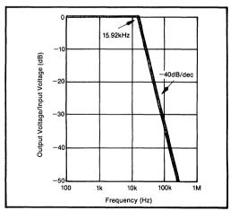
FIGURE 7. Linear First Order Approximation of Filter Circuit.
