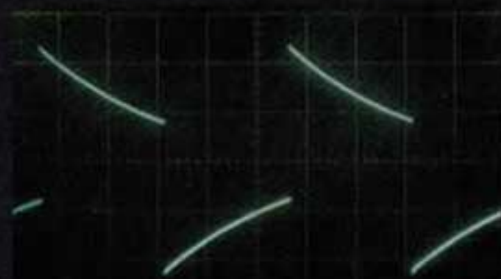
10Hz Squarewave Response: A Conventional Power Amp
